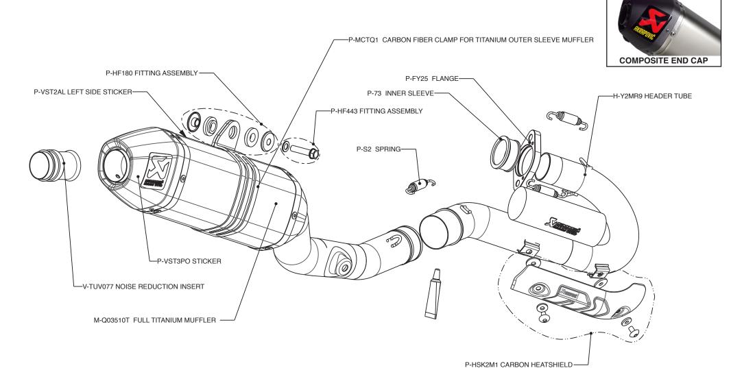
For the Racing system we use stainless steel tubes and composite end cap
