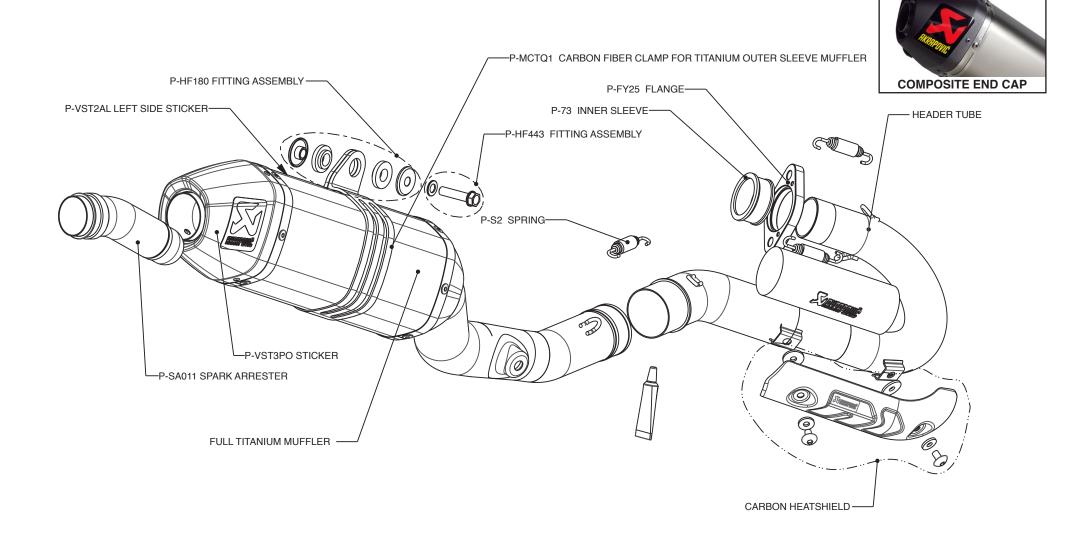
For the Racing system we use stainless steel tubes and composite end cap
